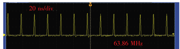
图 7 Tm:LYF 连续波锁模激光器的脉冲序列 Fig. 7 Pulse trains of the CWML Tm:LYF laser
